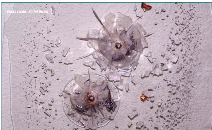
Ricochet Glass Product, all laminated test sample; glass deflecting bullets
