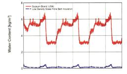
(Left) Moisture content of exterior sheathing with permeable air barrier— Chicago(CZ5).
