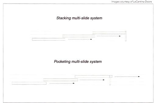
Multi-slide doors are classified by their different operation methods: stacking multi-slide doors and pocketing multi-slide doors.
