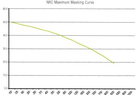
A sound masking spectrum or 'curve' is typically specified by an acoustician or supplied by an independent third party, such as the National Research Council (as shown), rather than by the sound masking system's vendor.
