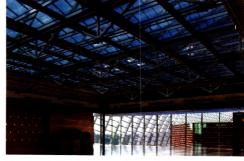
LEFT: The shape or form of a building can be used to optimize the exposure of interior spaces to use beneficial daylight. MIDDLE: Side daylighting is a legitimate strategy for bringing natural light into perimeter zones of a building. RIGHT: Top daylighting is an effective method to bring abundant natural light into interior building spaces.
