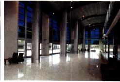
At Chabot College in Hayward, California, designers wanted to incorporate as much glass as possible to flood the interior with daylight and keep a connection to the outdoors. Electrochromic glass was used (clear on left and tinted on right) instead of mechanical shades or blinds in order to retain the view and keep the openness of the space.
