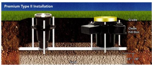
A Premium Type II installation further increases drainage on a project site by adding a subsurface perforated pipe, commonly referred to as a French Drain.
