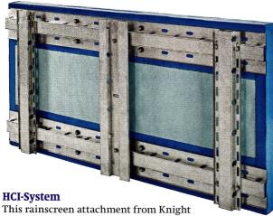
Wall System enables ASHRAE 90.1-compliant continuous insulation with numerous vertical cladding systems and materials (fiber cement, metal panels, aluminum composite material, etc.). Pre-assembled off-site, the system is ready to install at delivery and can span 32" on center. knightwallsystems.com circle 208
