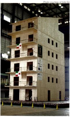
Seven-story CLT building being tested on the world's largest shake table in Miki, Japan
