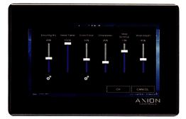
connects with mobile devices via Bluetooth, can manage up to 36 zones or can be wirelessly ganged with up to seven additional stations, to control as many as 288 zones. It can accommodate preset scenes, control movable fixtures, and manage intensity, color, and white-color temperature, among other settings. acuitybrands.com CIRCLE 214
