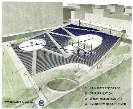
**BUSHWICK INLET PARK** The three-acre park (middle) on the East River waterfront in Brooklyn is designed so that no stormwater is sent to the city's sewer system. It was conceived as a blanket of turf that folds up to cover the roof of a wedge-shaped community building (top).
