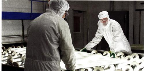
Inside a glass fabricator facility in Owatonna, Minnesota, an interlayer is applied during the laminating glass process.
