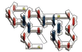
CORE STRENGTH The diagram above shows the blocks' shared cores. Red = two elevators, one stair; blue = two elevators, two stairs; yellow = one elevator, one stair.
