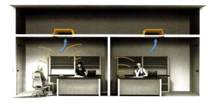
Plenum noise flanking is reduced by air transfer silencers.
