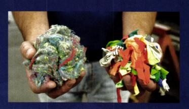
captured and used to create batt type insulation products with superior characteristics for use in commercial and residential buildings of all types. Recycled cotton textiles are also being used in various ways to create very effective acoustic insulation products or being integrated into other building product systems. We will take a closer look at these insulation products and their increasing popularity in the following sections.
