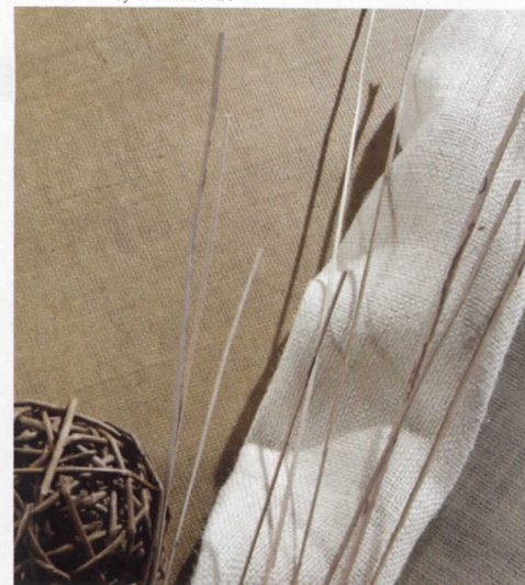
A burlap-textured, high-pressure laminate created originally for a chain of coffee shops was made by embedding a layer of jute textile between laminate layers.
