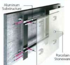
Cross-section of Marazzi's Ventilated Wall System
