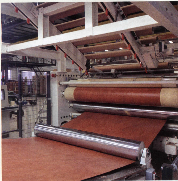
Natural linoleum is formed from a variety of rapidly renewable materials, including linseed oil, wood flour, and pine rosin (above left). During production, the ingredients are heated, mixed, and rolled flat (left). The sheets are cooled, backed with jute, then dried and trimmed. Pigments that do not contain heavy metals are used to achieve a wide variety of colors and unusual flooring installations (above right).
