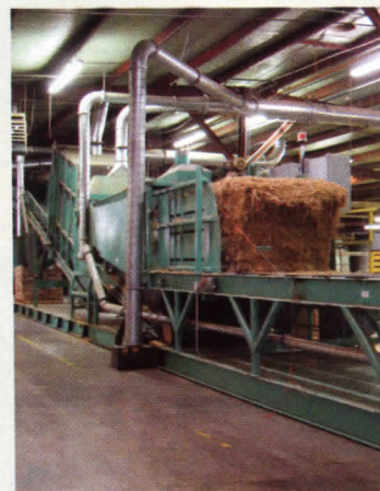
Oak Lodge (top left), a Jesuit retreat in California's Sierra Foothills designed by Siegel & Strain Architects, has walls of highly insulating straw bales covered by stucco. Details for incorporating the straw bale into standard construction (left) are evolving. Agriboard Industries subjects wheat and rice straw to intense pressure and heat as part of a manufacturing process (right) for panels (above) that provide structural strength and insulation.
