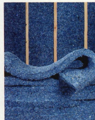
Cotton insulation (right) is produced with denim scraps from blue-jean manufacturing, diverting tons of material from landfills.
