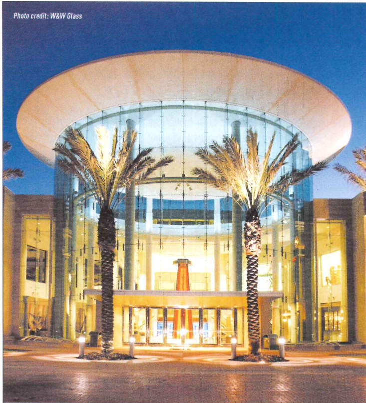
The Mall at Millenia, in Orlando, Florida, uses point supported bolted glass to maximize transparency between the outdoors and the indoor retail environment. Architect: JPRA Architects
