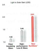
The Light to Solar Gain (LSG) value of SunGlass™ far outperforms high-performance solar control Low-E glass. The higher the LSG value, the better the glass performs at transmitting daylight and reducing heat gain from the sun.
