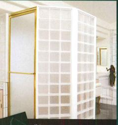
45-degree corner caps were used to connect Hy-Lite spanels to form this neo-angle shower. Flat caps were used to finish off the top and sides of the doorway, while a flat cap and mounting channel were used to attach the panels to the curb and wall.
