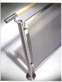
CIRCUM™ stainless railing system: Manufactured of corrosion-resistant stainless steel, CIRCUM is ideal for interior or exterior applications in commercial and residential facilities. Infill panels available in, but not limited to, perforated stainless steel, tempered glass, and stainless steel, tempered glass, and stainless steel rods. Handrails in wood/stainless, stainless, or colored nylon. Curved rails and custom designs are available. HDI Railing Systems. Email info@hdirailings.com
