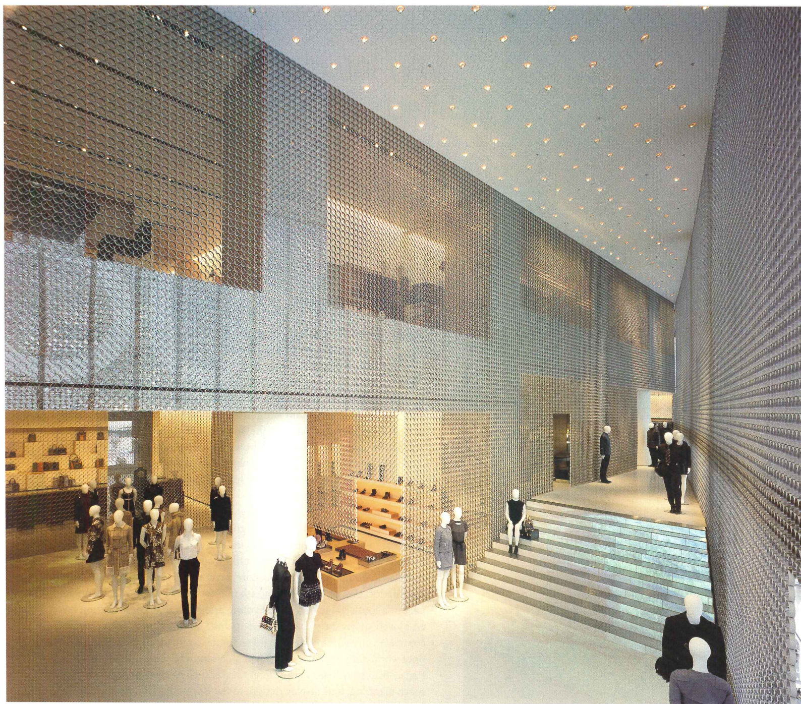
The architects wrapped the store's "nave" with an interior skin of metal rings and glass (above) and hung the same materials from the ceiling to create translucent partitions (right and far right).
