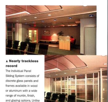
Sliding System is supported from a hidden track above the panels. As a result, of single narrow track is required for the floor; if weatherproofing is not a considered then trackless options are available. Panels can be stacked conveniently out of (top). The system is suitable for restaurants, stores, mall fronts, ski lodges, conference rooms, offices, and churches. 800/411-NANA. Nana Wall Systems, Mill Val Calif. CIRCLE 227
