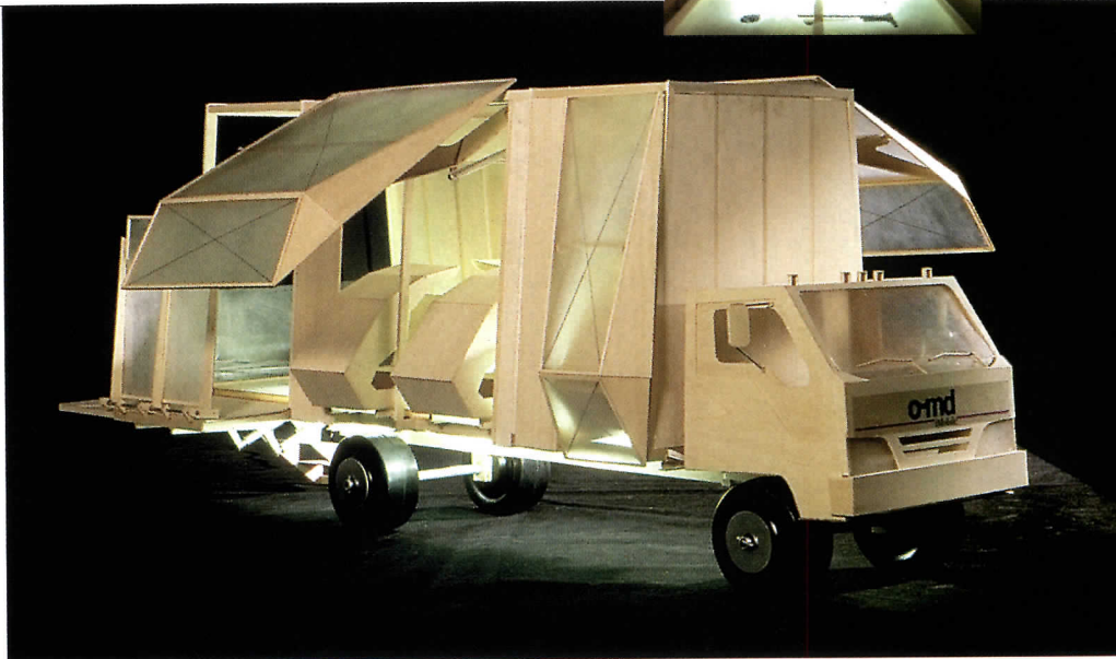
iMobile, unbuilt, 2000 Office of Mobile Design. The iMobile is designed to showcase new computer hardware and software or to provide computer access to schools, rural areas, or other locations where it would not otherwise be available.
