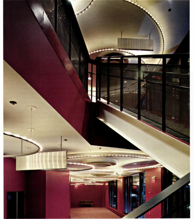
The theater vestibules and corridors showcase "halos of light." **Custom ceiling**mounted rings studded with low-voltage lamps are suspended at three heights to create a sense of movement. "The fixtures foreshadow the circular motifs inside the theater," Bettridge says. Additional halogen strips illuminate surfaces such as perforated-metal banisters.
