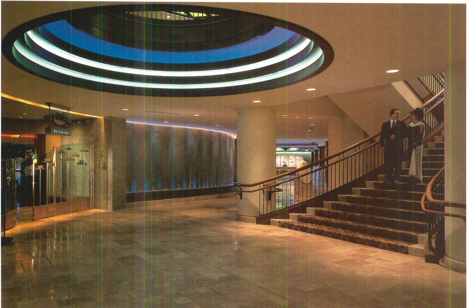
A ceiling mural is washed by uplight from 50W, 3,000K compact fluorescents mounted in side troughs (opposite). A valance
