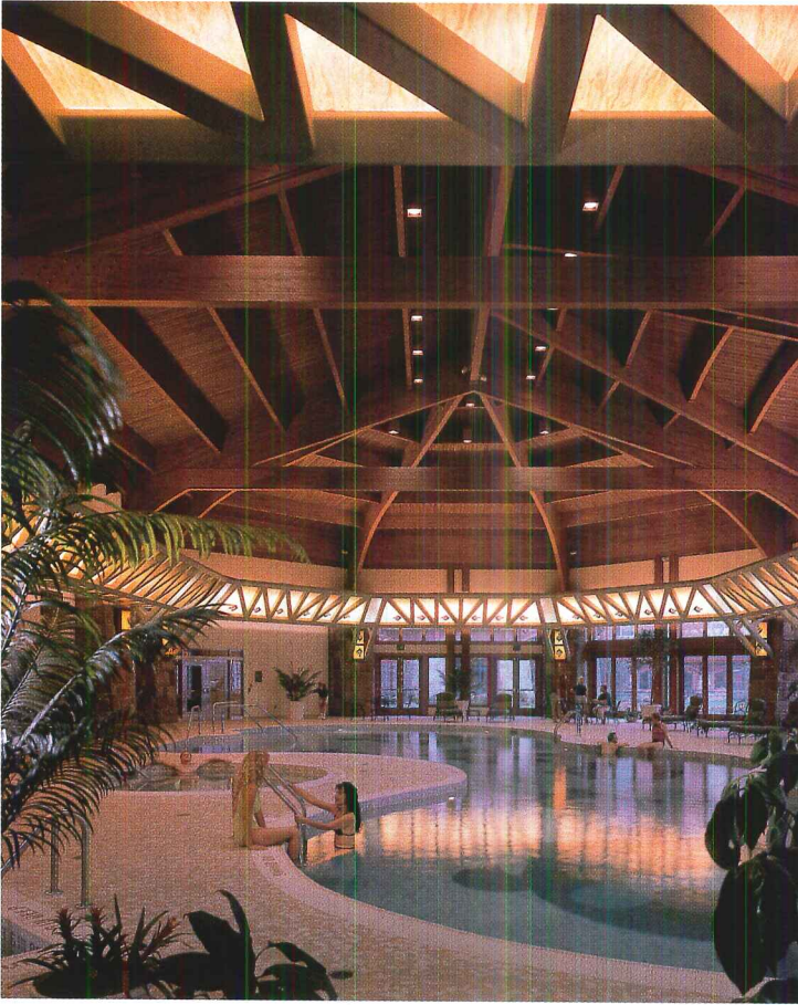
A ceiling mural is washed by uplight from 50W, 3,000K compact fluorescents mounted in side troughs (opposite). A valance
