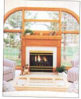
products have taken direct-vent technology & incorporated it into a new high performance fireplace. Model 6000 Supreme is a high efficiency fireplace (thermal efficiency up to 74%) & has an AFUE (Annual Fuel Utilization Efficiency) rating of 63%. The 6000 Supreme is standard with a variable regulator to adjust the flame & BTU input with the turn of a dial. Heat-N-Glo, 6665 West Hwy 13, Savage, MN 55378, 1-800-669-HEAT.
