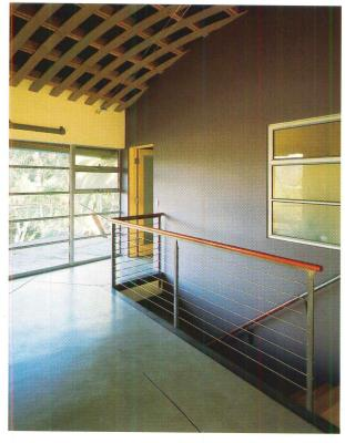
The "dog trot" (above), a transitional space that is enclosed but not air-conditioned, separates the public areas from a bedroom. The concrete wall of a stair (top right) was poured into a plastic-sheetlined form to give it an irregular surface.
