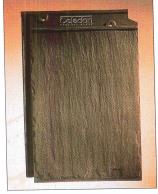
A kiln-fired, interlocking clay roof tile designed to look like thick slate with a breaking strength greater than 300 pounds; impervious to freezethaw degradation with less than 1% moisture absorption; color will not fade, flake, or effloresce-offered in slate gray, slate red, montpelier green, plumstone, and brunswick black. Sixty-year limited, transferable warranty.
