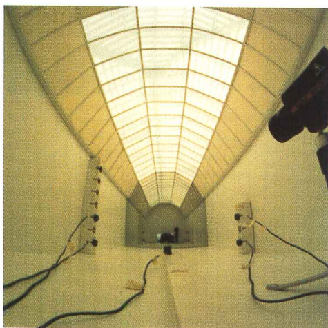
A model of one of the proposed MCA galleries (left). Rows of photometers are used to collect luminance data, and the video camera will be used to scan the model. The model itself (right) is very large.
