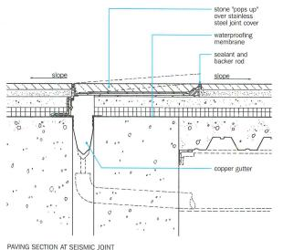
The Getty was constructed to high seismic standards. A pop-up stone paving panel avoids a metalplate cover over a drained 5-in. seismic joint (left).
