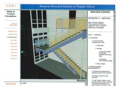
Seattle's NBBJ is experimenting with 3D design and construction documents on an extranet. Clients and contractors can view the design of a stair in a Lightscape-rendered image (below). Another model view associates specifications data (left); clicking on individual stair elements brings up further information (right).
