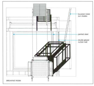
room open to the garden and street on all three of its exterior exposures. Mechanical louvered screens riding in angled, exterior tracks can be lowered to provide varying degrees of privacy, or raised to allow full views. In any position, they provide high-tech punctuation marking the end of the extension.
