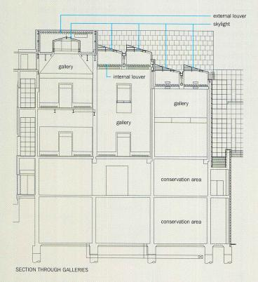
C/S prebuilt 17-in. louver sections as long as 17 ft (detail, top left). Lighting and photocells were set in a recess
