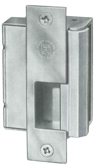
319. Remotely operated strike A new line, Series 600 electric strikes provide remote control of a swinging door: Made to fit narrow, 1 3/4-in. hollow-metal or aluminum jambs, strikes are compatible with many cylindrical, deadlock, or latching locksets. Stainless-steel devices meet UL burglary and fire-door (4 hour) ratings; available in fail-safe or non-fail-safe models. 708/739-3900. Folger Adam Co., Lemont, Ill.
