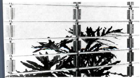
319. Clear security grille. For openings up to 45 ft wide and over 14 ft high, Vistaguard panel grilles allow full visual access while providing a solid security barrier. Lexan panels with aluminum rods form an almost airtight construction so grilles can separate air-conditioned spaces in retail malls. Cornell Works, Inc.
