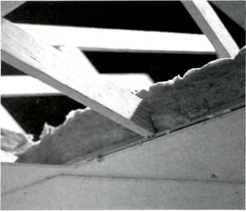
317. Fire-rated assemblies. FR-Quik Channel Sets permit the use of structural wood trusses and I-beams in insulated floor and roof systems in occupancies that require two-hour ratings. Acting as an edge block, the channels maintain the integrity of gypsum panels during fire exposure. Lumbermate, Alpine Engineered Products.
