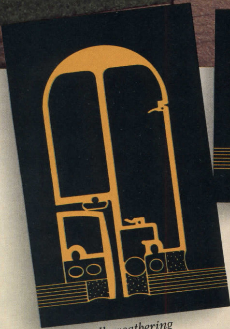
Sealair bulb weathering to reduce air infiltration at door perimeter.
