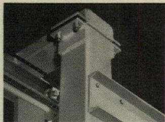
Shims simplify track leveling.
