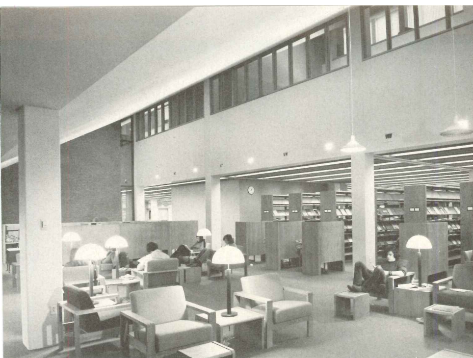
High-intensity quartz lamps wash the sloping ceilings with light.
