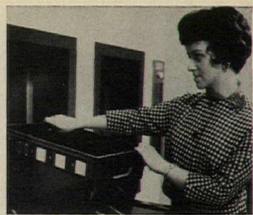
At proper floor, the box is automatically shunted off vertical conveyor. "Magnetic memory" control system has no moving parts, levers, or between-station wiring... nothing to wear out.
