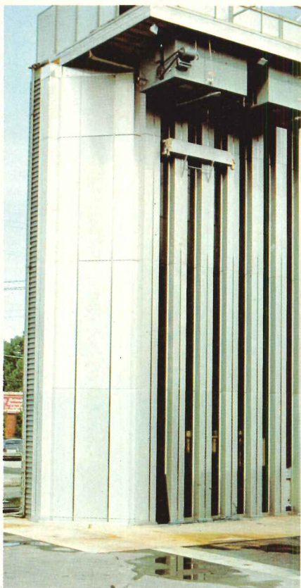
(Left)—Testing a prototype of the wall system by Cupples Products Division, H. H. Robertson Co., checked out the wind loading and thermal performances.
