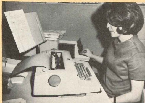
Magnetic tape drives IBM Selectric typewriter at 150 words per minute for error-free specifications in copy reproducible by offset.
