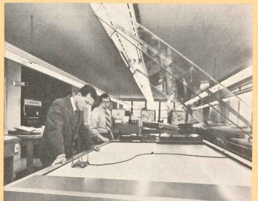
Xynetics, computer-plotter (above), is the $100,000 draftsman now at work for Saphier, Lerner, Schindler, Inc. planning space for the new Sears building in Chicago.
