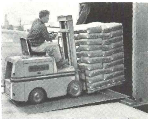
Torsion bar actuated hinged lip dock leveler
