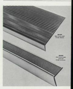
STAIR ACCESSORIES / Friction-Grip's nosing and tread design consists of closely-spaced pyramidal points. The double row of grippers on the tread affords protection where maximum wear and potential danger lie. The corrugations run full depth and have no dust-collecting crevices. The nosing needs no metal strips. Made of resilient, wear-resistant vinyl, both the tread and nosing are available in several colors. The Mercer Plastics Company Inc., Newark, N.J.
