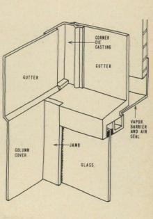
The cut-away detail above shows the flashing gutter, which is continuous around the entire building at every floor.
