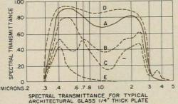
When solar radiation strikes a sheet of glass it is either reflected, transmitted or absorbed. Chart compares transmittance of various glasses, including special glasses available with low transmittance to the sun's infrared heat.
