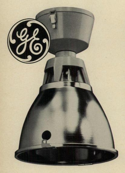
New activated charcoal filter keeps dirt away from lamp, reflector and inside door glass. Even enclosed luminaires "breathe" air in and out through natural expansion and contraction of the air inside. But the filtered optical assembly in Filterglow fixtures permits the entrance of cleaned air only. The results: an absolute minimum of efficiency-reducing dirt build-up inside, better maintained light output, and less frequent cleaning.
