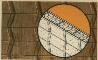
BLOK-LOK® or THIN JOINTTM for horizontal reinforcing in masonry walls
