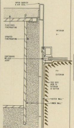
The horizontal section above shows how the pressure equalization theory is adapted to glazing.
