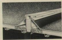
In addition to protection from cracked felts along the water dams, the expansion joint provides safeguards against leakage into the joint itself. A vinyl strip at the bottom, from one roof edge to the other, moves with the roof to form a positive, continuous seal. The extruded aluminum sides and related components, being free-floating, are also independent of thermal reaction between the water dam and felts. Transitions and injunctions are factory fabricated. are factory fabricated.
