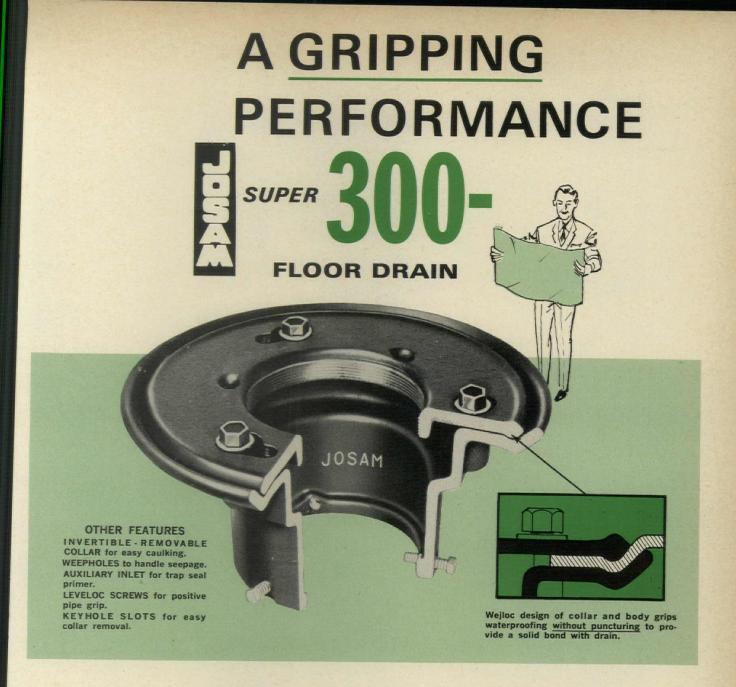
The Josam Super 300- Drain has several important features that provide a superior installation. The Wejloc design on the collar provides a positive NON-PUNCTURING bond of waterproofing to drain. The heavy threaded collar provides a choice of Josam adjustable strainers including the Type ASF Super-Flo strainer (more sanitary, stronger, and drains water faster.) The Super 300- drain is designed to meet the requirements of modern construction. Specify them on every job. Write for Manual TJ today.
