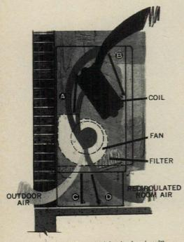
Dampers C and D control fresh air mix with room air. Face and bypass damper (A) regulates air flow through heating/cooling coil. Exclusive Modine anti-wipe damper (B) reduces heat pick-up from coil to 5% when heat is not needed.
