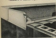
ss section from Sweet's, shows how the free-floating interlocks with, but moves independently of, the galvanized steel water dam. The graceful fascia profiles are available in Kalcolors, porcelain
