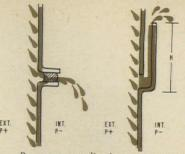
Pressure equalization to prevent leakage stems from the following observations: difference in pressure from wind loads sucks water through tiniest openings (above left); flashing gutters do not prevent water build-up under constant pressure differential (above right).
