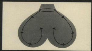
This drawing shows how a diffuser moves air unevenly. The air shoots out, much like through the nozzle of a garden hose. Sit under one of the blasts, and you'll know what we mean. Air can stagnate in one area of the room, and drafts build up in the other.
