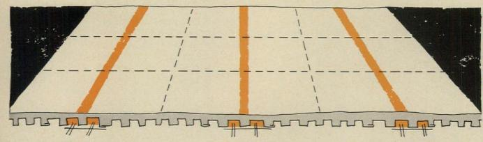
Things have changed. Inland Hi-Bond Celluflor and floor deck are now available in such a wide range of profiles that you can match electrification and building modules simply by blending the cellular and non-cellular steel panels.
