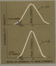
The smaller the coefficient of variation, the fewer lights of glass would have a given percentage of strength less than the mean. A figure of 42 per cent less than the mean is used in the probability curves top left as an example. The two lower charts show how both the coefficient of variation and the total number of lights in a building change the required safety factor.
