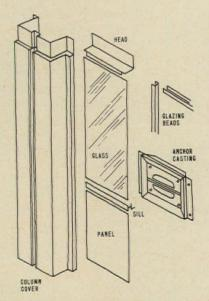
The basic standardized components which assemble to form the curtain wall are shown in the diagrammatic sketch above.
