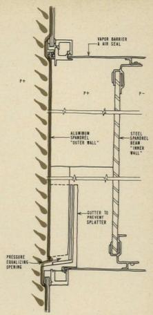
The World Trade Center curtain wall spandrels use steel structure as inner wall to achieve pressure equalization.
