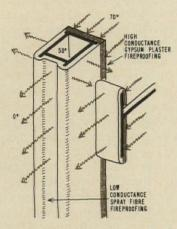
The heat flow characteristics of column, spandrel and fireproofing are shown in this diagram.
