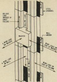
The metal curtain wall is designed to resist total design loads and transfer them into the building frame. Direct wind loads on washer and wall are not considered additive due to air voids between them.
