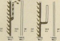
A pressure tight inner wall equalizes pressure, but too large a void, combined with narrow air path (above left) still permits overspray. A smaller void and wide air path (above right) help by giving immediate equalization response. Wide aperture reduces air velocity and stops overspray.
