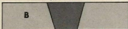
Figure B, however, shows how a joint can deviate from design during construction.
