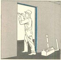
**Installation**—Aluminum frames are installed after wall construction is complete and the trades involved—even painters and paperhangers—are finished. Scheduling is simplified. Frames are free from damage.
