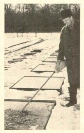
Test plot at PCA laboratories shows how air entrainment prevents scaling. Slabs containing 6% entrained air (left) show no scaling after five winters of severe exposure and heavy salting. Nearly all of the non-air-entrained slabs (right) have scaled. For further details write for free information sheet, "Air-Entrained Concrete." (U.S. and Canada only.)
