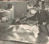
HIGH COVERAGE, MINIMUM LABOR! Using 3M-recommended spray system, a gallon of Insulation Adhesive 33 effectively bonds about 600 square feet of duct liner. Open time of 5 to 7 minutes permits spraying large areas quickly, conveniently.
