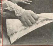
IMMEDIATE TACK. Right-now strength. Here, just seconds after the bond was completed, the insulation delaminates, but the adhesive holds tight. It continues to hold tight even after extensive aging at high temps, does not become brittle.
