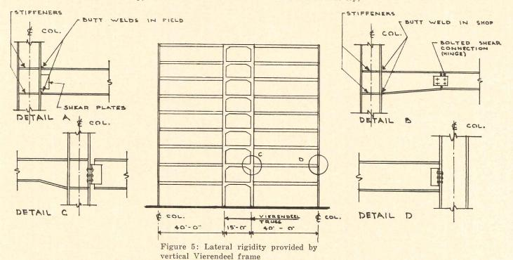
STABILITY BY VARIATIONS IN CONTINUITY. The use of braced bents, though providing rigidity with economy, may limit the flexibility of the floor plan. Continuous rigid frames (Figure 3) offer nearly the same resistance to lateral loads, with the added advantage of reduced depth of construction. Frame action is obtained by making the connections of all beams to their supporting columns rigid, i.e., non-rotating. These must be made in the field at a higher cost than standard bolted connections.
