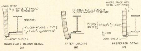
Figure 4. Masonry bends due to flexible clip. Stiff connector precludes this
