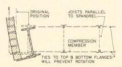
EXTERIOR SPANDREL BEAM Figure 5. Ties needed between joists
