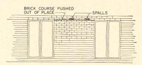
Figure 2. Ice forms at spandrel beam; cracks wall
