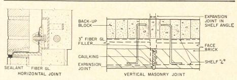
Figure 16. Horizontal joint
