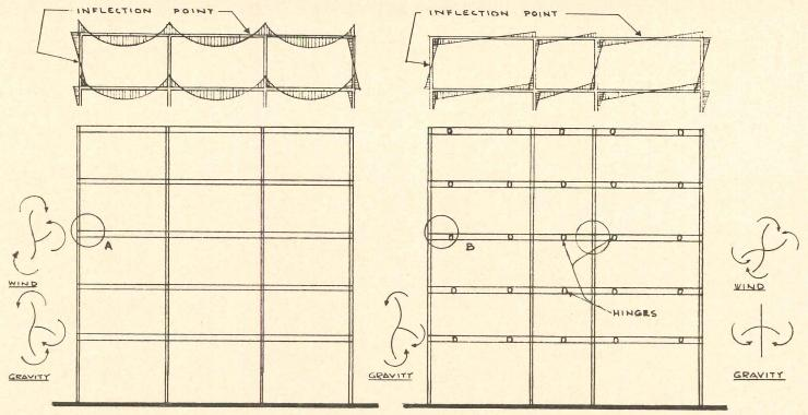
Figure 3: Continuous frame (gravity load moments shown at top)
