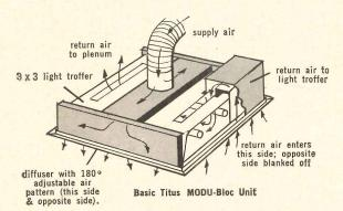
A ceiling air diffusion system and complementary ceiling suspension system that provide the maximum in efficiency, flexibility and economy in integrating SOUND AIR DIFFUSION, good lighting and acoustical control.
