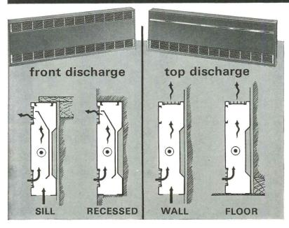
The only electric convection heater that gives you a choice of air intake — front, bottom or both—and heated air discharge—through the front or top. It is available in lengths of three and four feet, heights of 11, 15 and 20 inches, and depths of 3, 4, and 5 inches.
