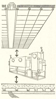
The Inland Radiant Comfort System is made up of three basic components, carefully engineered to work together more efficiently than any one of them could work alone. The components are not new to architects and mechanical engineers. They are: (1) a radiant-acoustic ceiling, (2) a chemical air conditioner, (3) a cellular steel floor (optional in hospital construction).
