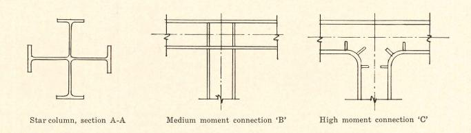
MINIMUM COLUMNS AT TYPICAL FLOORS. Special conditions of design may demand column free areas on all floors of a tall building. Floor beams may span the width of the structure if composite action is established between the beams and concrete slab. Carrying girders may be Vierendeel trusses as shown in Figure 9. Triangulated trusses or plate girders with the accompanying disadvantage of window restrictions may also be utilized. Regardless of the type of
