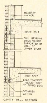
Figure 3. Shelf angle not firmly attached
