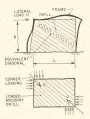
Figure 9. Masonry partition too close to structural frame
