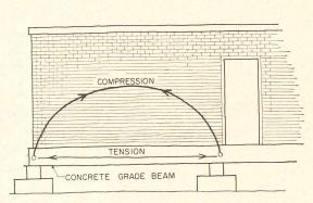
Figure 8. Rigid masonry acting as a compression arch
