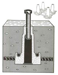
without any awkward projection of bolts. Typical applications include bridge railings, building columns, signs and light posts. The system is available in ½, 5%, ¾, 7%, and 1 in. bolt sizes. Decatur Engineering Company, 519 East William St., Decatur, Ill.
