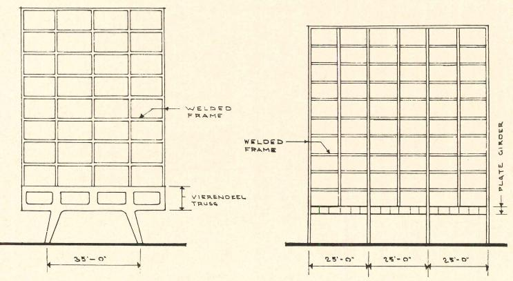
Figure 7: Vierendeel truss forms transition frame at first floor
