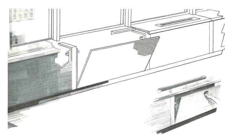
What do you call a foam-filled under-window enclosure that snaps into place with magnetic locks that eliminate knobs, keys, bolts, screws or slots...comes in a wide range of finishes including aluminum, plastic and steel... will not warp, buckle, bend or vibrate...and weighs only 2 lbs. per square foot?
