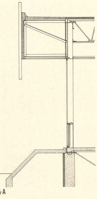
The structural peripheral wall is of aluminum and glass, with suspended precast panels—of plastic cement with white quartz aggregate—serving as sun breakers. Aluminum mullion-columns are a special extrusion designed by the architects; note how they are adapted to turn the corner. Clear plate glass is set in vinyl glazing channels above the sill line; gray-coated glass below
