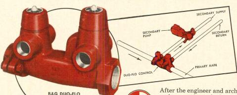
In Primary-Secondary Systems equipped with B&G Duo-Flo Controls, secondary zones are always positively controlled, even with high head primary pumps. Use of higher temperature drops permits sizable reduction in pump horsepower. A Duo-Flo Control eliminates 2 Flo-Control Valves, 2 shutoff valves, 2 or 3 tees and 6 nipples.
