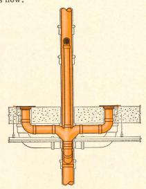
SAVES BETWEEN-FLOOR SPACE. In this layout, the use of compact, space-saving copper for the sanitary drainage system saves  $5\frac{1}{2}$ " of building height per floor. In a multistory structure, this could mean thousands of dollars saved in construction materials and labor.
