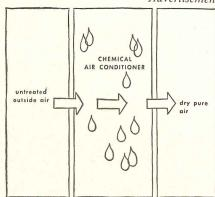
Chemical air conditioning removes the latent (humidity) load from incoming outside air. A non-vaporizing solution of lithium chloride with a great affinity for moisture is sprayed into the air stream. Condition of the air as it leaves the dehumidifier at a specified humidity level depends upon (1) solution concentration and temperature, and (2) temperature of cooling tower water.
