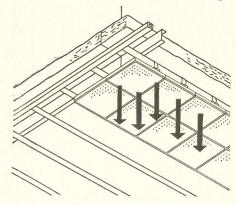
The radiant-acoustic ceiling acts as a single, wall-to-wall heat exchanger. Heating and cooling are accomplished by means of aluminum panels attached to grids of water pipes hung in the manner of a conventional suspended ceiling. Hot or cold water is circulated through these pipes to heat or cool the panels. Heat loss and noise are reduced by an acousti-thermal blanket.
