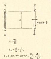
Figure 6. Derivation of rigidity ratio
