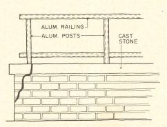
Figure 14. Cracking due to railing expansion
