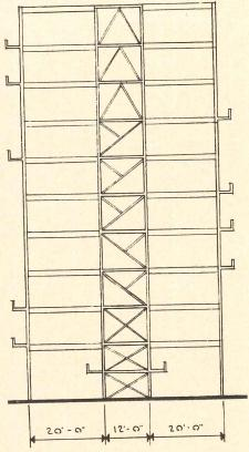
Figure 1: Variations in braced bents to permit corridor and door openings
