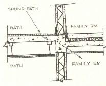
If different construction types are flanked, impact noise from the "poorer" construction will travel through structural slab on the floating floor side
