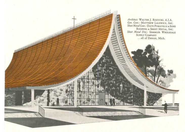
In conceiving the design of this structure the architect, Walter J. Rozycki, visualized the bold, soaring sweep of the roof as the commanding element of the overall structure, both in size and contour. Said he, "Such a roof, without the use of copper and its characteristic design flexibility, would have been virtually impossible."
