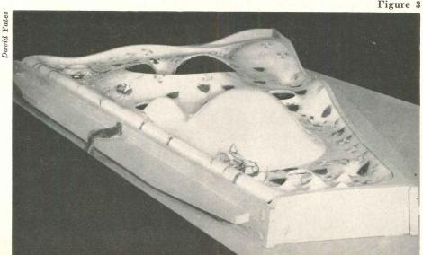
Display model of the Eastman Kodak pavilion for the 1964 New York World's Fair is shown in Figure 2 (above). It literally is a free-form shape, made up of many shell shapes, few of which could be expressed accurately by mathematics. The structural model in Figure 3 (left) was used to provide stress patterns and column reactions. Designers. Will Burtin, Inc.; architects, Kahn & Jacobs; structural engineers, Lev Zetlin & Associates
