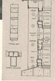
Typical wall section with LUPTON Curtain Wall
