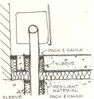
Pipe penetrations are sleeved and packed to prevent the impact noise from being carried through the pipe
