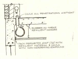
All penetrations must be caulked to prevent transmission of impact sound through piping, ductwork; also to stop airborne sound (above). Conduit and duct connections must be flexible to maintain impact noise reduction of floor (below)
