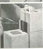
Strength with flexibility—the two basic factors for a repair-free masonry wall are assured by these engineered companion products. Dur-o-wal reinforcement, top left, increases the horizontal flexural strength of 8" concrete block walls from 60 to 135 per cent, depending on the weight and spacing of Dur-o-wal used, and type of mortar. The ready-made Rapid Control Joint, beneath, with its neoprene compound flange, flexes with the wall, keeps itself sealed tight.
