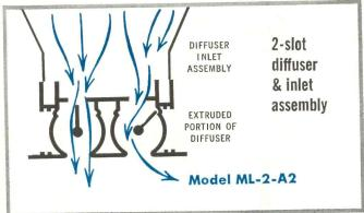
Air pattern controller, in both models, adjusts air flow a full  $180^{\circ}\dots$  Patent applied for
