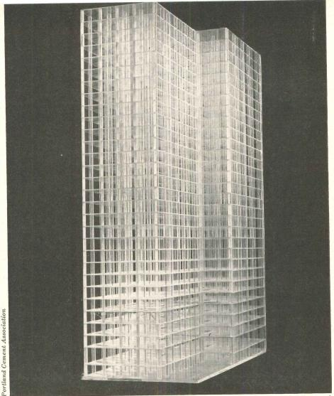
Tests on the model of a 29-story flat plate structure for Carl Sandburg Housing in Chicago (Figure 4, left) indicated that 15 per cent less slab reinforcement was necessary than mathematical analysis showed. Also shear wall size and location was based on the structural model analysis. Cost of the model analysis was about 15 per cent of the savings it made possible.
