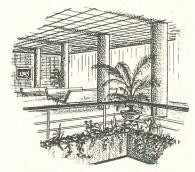
Used in, or adjacent to glass walls, round columns offer minimum obstruction to light and occupy minimum space for a brighter interior.
