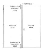
New Weldwood Fire Doors hung in pairs, Class "C" label, ¾-hour. Maximum size opening 6' x 7'. Astragals and Glenraven surface bolts supplied with doors, but not attached.
