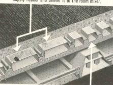
These standard size structural cells can carry wiring for power and communications of all kinds.
