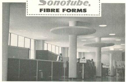
In any structure where round concrete columns are planned, SONOTUBE Fibre Forms will usually cut costs. In your next design, specify SONOTUBE Fibre Forms—fastest, most economical method of forming all types of round concrete columns.
