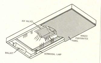
chamber is completely exposed to high-intensity rays emitted from the germicidal lamp and then evenly distributed into the room through perforated metal panels. The Pyle-National Co., 1334 N. Kostner Ave., Chicago 51, Ill.
