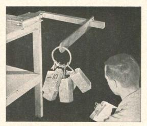
**Dual-Moment Lever Arm and Torque Test...**Simulates the most common, failure-causing loads submitted on door corners.
