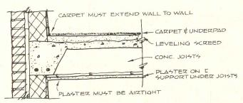
Plaster must be airtight to get most loss of energy through the structure and to prevent transmission of airborne noise
