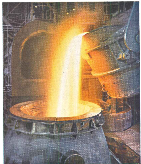
Charging molten iron into the vessel.
