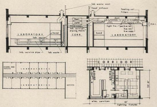
Typical layout for center corridor with labs on each side can provide office cubicle or desk space in laboratory area or adjacent wing depending on whether proximity to work or isolation for study is predominant factor. Mechanical services shown in section at top are similar on each side of corridor. Details suggested may vary
