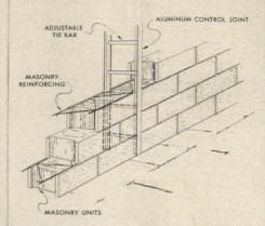
use of different size and type masonry units without keying. The joints are adjustable for any wall thickness and can be used for both interior and exterior applications. *United Areo Products Corp.*, Burlington, N.J.
