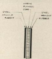
riors of the door bonded to the steel. A full-length rubber hinge permits full openings in either direction and eliminates need for lubrication. Clark Door Co., Inc., Rose St., Newark 8, N.J.
