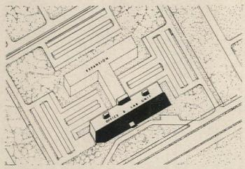
The single structure laboratory and office unit is well adapted to research programs of definite or limited objective and to a restricted site. It provides internal flexibility, but expansion may be costly or disruptive
