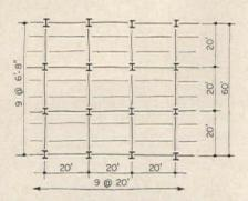
Figure 3: In conventional framing for a 60-ft module, columns are on 20-ft centers; beams are 6 ft 8 in. apart
