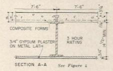
Figure 1: Actual beam depth depends on load. Minimum depth of 14½ in. is required for fire-resistance rating
