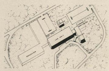
The articulated plan is a reasonable compromise between the single building and campus plans, permits isolation of hazardous operation, but may develop problems in service distribution and communication between add-on related units
