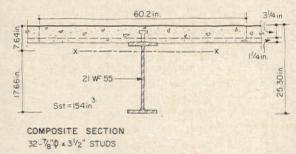
Figure 6 (above): Design for composite section which will satisfy dead and live load moments
