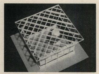
Model shows roof framing and simulator placement
