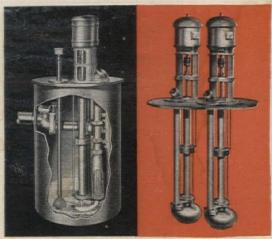
Flush Kleen Clog-Proof Sewage System Capacities to 1000 GPM, Heads to 105 Ft. Bulletin 122D
