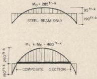
Figure 5a: Bending moment for 60-ft beam due to the dead load
