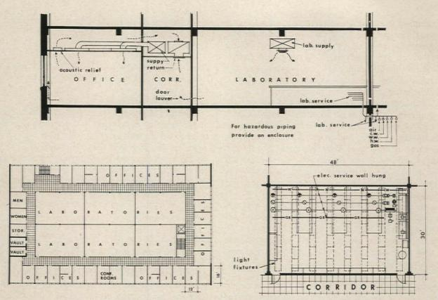
3 Core laboratories with perimeter offices make a layout suitable for large establishments, especially in "dry" research, where flexibility in lab areas is required. Service distribution to labs is relatively simple near center wall. Zoning of air handling systems is also fairly simple. Details are optional
