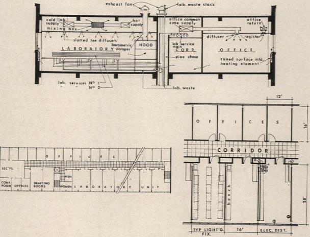
Off-center corridor with offices on one side and labs on the other provides extra office space for theoretical physical research. Hood exhaust for contaminated work would be vented far from any intake. Narrow doors between labs might be provided at outside wall. Electrical requirements may be extensive and cooling loads may be high
