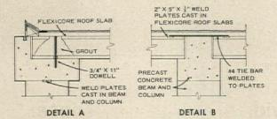
New Hi-Stress Flexicore slabs use high-tensile 7-wire stressrelieved strands to produce fully prestressed units. These slabs provide long, clear spans, high load carrying capacity and give improved performance.
