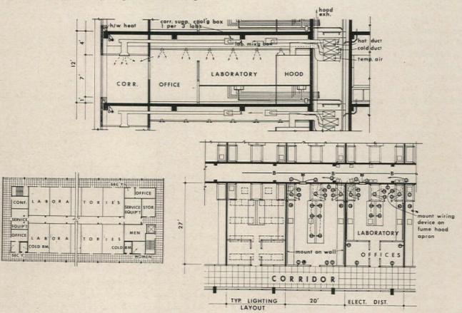
Perimeter corridor with interior laboratories separated by mechanical service passageway provides easy access and flexibility for changing service requirements. Traffic and communications may be cumbersome, and workers' views of outside are limited unless privacy is sacrificed by interior window wall
