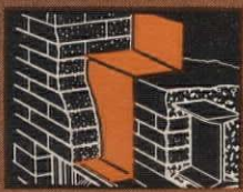
Spandrel beam waterproofing
