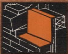
Window sill flashing
