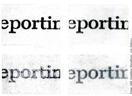
Veiling glare makes it harder for a person to see a task; this is caused by specular (mirror-like) reflections of the light source. These photos show the effect of different directions of non-polarized light. Viewing angle is 25 degrees. Top left: 90 degree incident light (perpendicular to paper); top right: 40 degree incident light (50 degrees from perpendicular); lower left: 65 degree incident light; lower right: 5 degrees incident light
