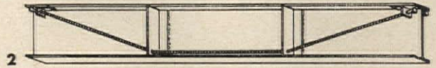
Fig. 2. High strength strand in beam web has effect similar to that of truss rod
