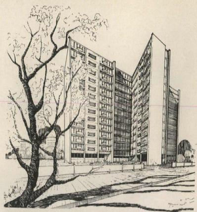
The 14-story structure, containg 104 two-and three-room units, is built in the shape of an irregular cross. The rear wall of each wing is solid masonry, without windows; as visual contrast, the front walls are almost entirely of glass, relieved by the horizontal lines of balconies containing planters.
