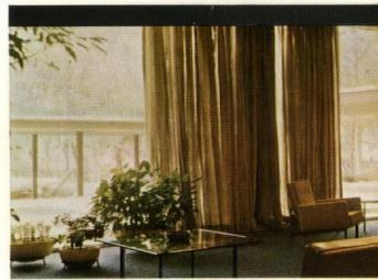
TOPAZ PLATE GLASS. Fine, integrally tinted plate was specified for all windows in GEICO's main building. This glazing takes full advantage of the wooded and landscaped site . . . transmits remarkably true color, yet cuts glare appreciably. From the exterior, the topaz tint becomes more apparent, the fenestration more opaque. The effect is rich and pleasing, helps to unify the window areas.
