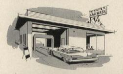
Drive-through—"OVERHEAD DOORS" front and rear (or front and sides) are frequently used by auto service centers, garages, car wash businesses and delivery companies to allow cars and trucks to drive through and avoid interruption of incoming and outgoing traffic.
