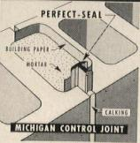
Williams "Perfect-Seal" (Pat. Pend.) is a specially designed seal for use in Michigan Control Joints . . . it provides continuous six-point pressurecontact sealing which keeps moisture out of joints and prevents air passage. The T-Section is a high-grade rubber compound; the cross-sealing member at the base of the "T" is a strip of readily compressible, nonabsorbent, expanded closed-cell Neoprene Rubber—it provides an effective pressure-contact seal directly behind the calking.
