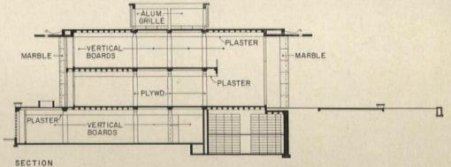
The building is sited over a former city street about 12 ft below the upper campus level. This grade differential was used to advantage by locating the entrance at the mid-level between the ground and mezzanine levels. The main floor is 150 ft long and 75 ft wide, the mezzanine is 150 ft by 52 ft, and the lower level is 200 ft by 100 ft. The total area is 40,000 sq ft
