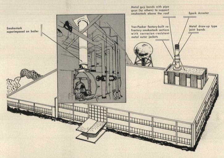
The Van-Packer Model HT Smokestack is the only industrial stack listed under the Factory Inspection and Label Service Program of Underwriters' Laboratories, Inc. It handles boilers, furnaces and incinerators. Van-Packer Smokestacks consist of factory-built 3-foot refractory sections with corrosion-resistant metal jacket and fittings. They cost
