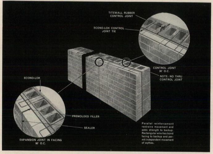
Exposed sides and interior sides of faced masonry walls are subject to differing stresses under varying atmospheric conditions.
