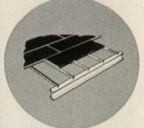
Tectum Box Section Roof Deck Assembly combines roll formed subpurlins and Tectum planks for speedy erection, lateral strength.
