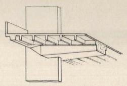
The basic structure is a deep, thin column, a wide, shallow beam and a ribbed slab. Theoretically the beam could be attached to the column in several ways. Below are the engineer's sketches and comments showing his approach to the problem. Structural behavior of the full frame is shown on the next page
