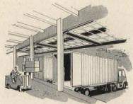
Reverse opening—"OVERHEAD DOORS" that open outward, rather than inward, follow the contour of outside wall and canopy. Their reverse opening provides needed head-room for fork-lift trucks and similar equipment used inside to speed materials handling.
