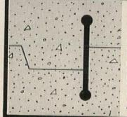
Williams Waterstops are made from Natural Rubber Stock and designed for maximum effectiveness in any type of cast-in-place construction joint. They will bend around corners, and will not crack or tear from shear action. Tensile Test: 3990 lbs., Elongation Test: 650%. Available in rolls up to 80 feet in length. Field splicing is simple. Williams Waterstops can also be furnished in Vinyl or Neoprene for industrial uses where resistance to oil and other injurious wastes is desirable,
