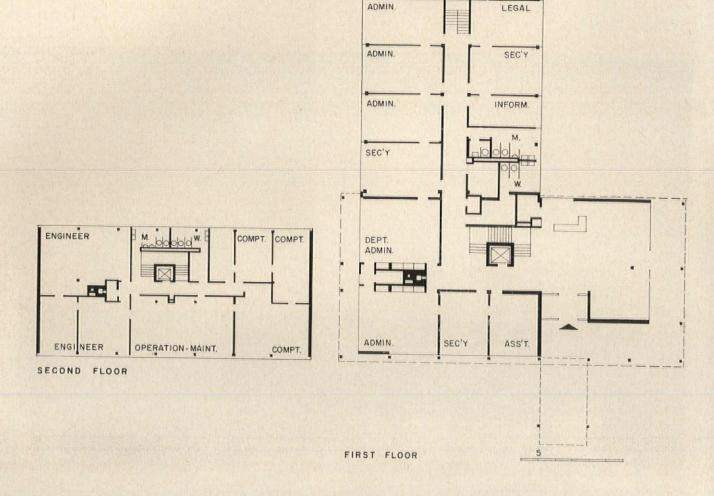
This three-level structure provides work space for men in charge of the construction of the St. Lawrence Seaway. Built on a site which slopes sharply to the rear, the basement extends toward a lower grade level of the slope and obtains natural light for additional office space at the rear. The first floor is occupied by administrative offices with a small exhibition lobby to the right of the entrance. On the second floor are engineer's offices and drafting rooms.
