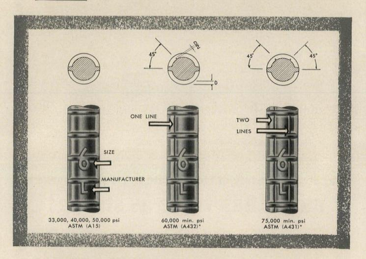
Standard high strength steels\* permitting greater economy and efficiency in reinforced concrete design under the provisions of the new A.C.I. codes must be identified. Recognizing this need, each Laclede Multi-rib reinforcing bar can now be completely identified as to size, strength and origin through a new rolled-in marking system. This assures the designer, contractor, and code writer that the proper grade of reinforcement is used on the job.
