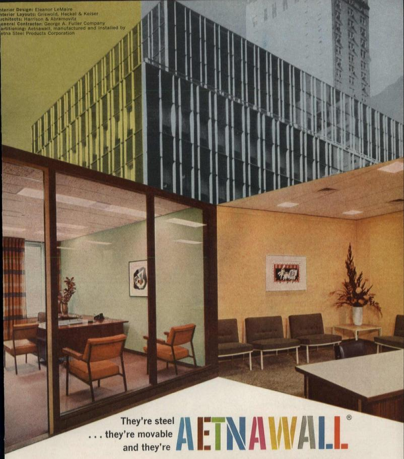
IN NEW YORK'S C. I. T. BUILDING, Aetnawall appears in many forms: floor-to-ceiling walls that look like masonry, as in reception area at right; framing members with full glass panels, as in supervisor's office at left; less-than-ceiling-height space dividers, and other wall treatments employing a variety of materials, textures and colors.
