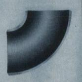
The unique shape of the HUSKY elbow is shown here. It results from cold-flow working which compacts the metal for enormous strength, while still maintaining the minimum wall thickness specified for Schedule 40 pipe. Note, also, the heavy build-up of metal in the crotch of the elbow . . . the point of greatest stress in piping.
