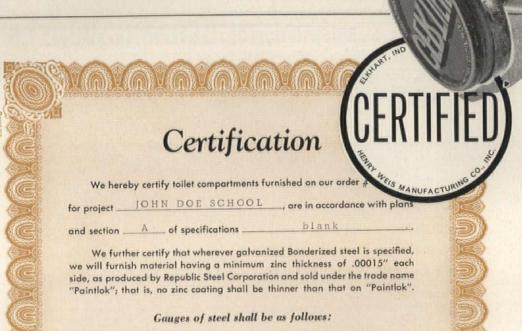
Flush Partitions of over 48" - 20 gauge Flush Partitions 48" and under — 22 gauge Panel Partitions of over 48" — 16 gauge Panel Partitions 48" and under — 18 gauge Stiles (with headrail) — 20 gauge Stiles (without headrail) — 16 gauge
