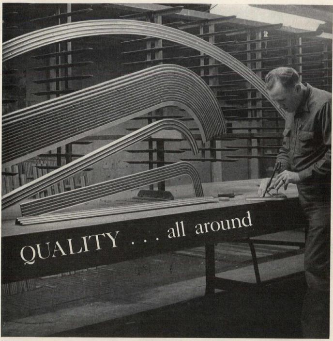
The curving of Wooster Super-Grit and Safe-Groove Safety Treads is just one of many exacting operations necessary to meet specific requirements of our customers.
