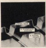
TOUGH FINISH. Rust-preventive enamel is "flow coated" over steel, baked on at 350° F. for 20 minutes. Flint-hard finish prevents corrosion, resists abrasion from field handling.
