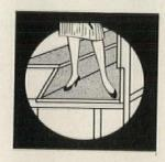
This is just one of the hazards eliminated by Hussey's safety-minded engineers who designed Closed Deck Roll-Out gym seats. The floor boards and front and rear risers are all one integral unit. There is no need to check footing because there is 16" to 18" of completely enclosed footboard. There is no opening for an accident.
