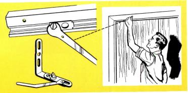
Simple door adjustment. Tighten or loosen single nut on top socket and bottom jamb pivot. Doors can be adjusted from either side, even when fully closed. Eliminates old "repeated adjustment" routine. And doors fit closer to jamb!
