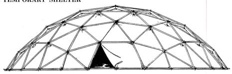
A 1300-lb aluminum and plastic dome, 57 ft. in diameter, is designed as a reusable, demountable warehouse, barn, salesroom and silo. The dome is constructed of aluminum struts with a non-rigid, seamless plastic skin, and, according to the manufacturer, can be put up or taken down in eight man-hours. The cost is \$3,750, FOB Mechanicsburg, making \$1.50 per square foot, exclusive of construction. Capitol Products Corporation, Mechanicsburg, Pa.
