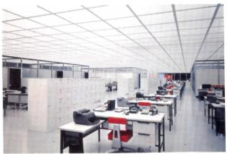
Flexibility of the Reynolds offices is obvious. Partitions can be easily moved to expand or decrease the size of various areas, whereas the Curtis wall-to-wall ceiling of light supplies 75 foot candles of maintained illumination. Curtis grid system is mounted 10 ft. 6 in. above floor level, with lamps spaced the new center. Here! Hopevite aluminum diffusers complement the decor.
