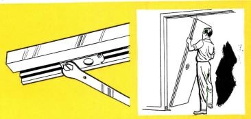
To remove doors, loosen just one nut on top track socket. Slide toward center. Top pivot and guide slip out of track. Just lift door off bottom pivot and away they go for painting, etc. Fastest, simplest removal ever — and from either side!
