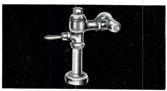
SI-FLO® quiet operating flush valve eliminates water hammer, line throttling and closing noises. Easy installation with  $36''\pm a$ djustment in 434" roughing; only one moving part; external adjustment controls water volume.
