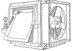
Figure 1. Draft inducer is a motor-driven airfoil fan in a metal housing
