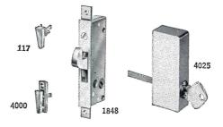
The 1848 Sliding Wall Deadlock shown above measures only 3%'' x 1%'' x 1%'' x 1%'' has a collapsible bolt for protection of door and lock, and operates with positive "feel appeal". To compensate for possible misalignment of door and jamb, bolt projection can be adjusted a full %'' by simply turning a screw in the lock face. The 4025 cylinder group is a clean-lined outside pull, offering key control that can be keyed-in with most popular cylinder systems.
