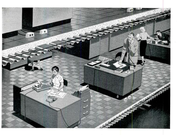
In 1957, Granco introduced a totally new method of providing raceways for electrification, plus reinforcing and forming of floor slabs—all in one operation!
