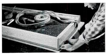
**Tight Seal** is assured by carefully applied gasketing. Gasket is soft sponge rubber resistant to acids, oils and greases.
