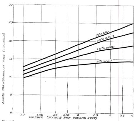
The relation between sound transmission loss and the mass of a folding partition as it is affected by sound leakage through cracks
