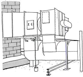
Figure 4. The inducer may be mounted at beginning of the breeching  $% \left( 1\right) =\left( 1\right) \left( 1\right)$
