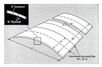
Prefabricated roof vaults are 11 feet wide at the chord, and 56 feet long (40 foot span plus 8 foot cantilever both ends). Key to system is the outstanding shear strength of the stressed fir plywood skins.
