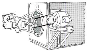
$Figure\ 2.$  Combination motor-driven and turbine-driven inducer can operate on steam, when power fails
