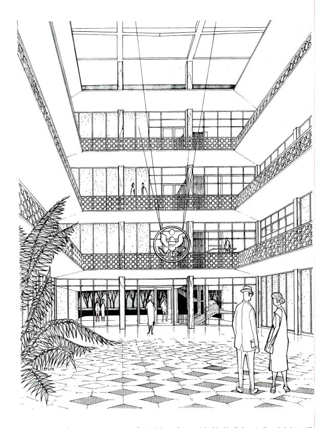
Balcony rails and pavement pattern are derived from that used in Marble Palace in Bangkok but will be of local pressed marble chip tile. Central court forms main reception area for visitors, arriving on foot or by car, with elevators to offices on upper floors at rear toward *klong*. Suspended from roof is Great Seal of United States
