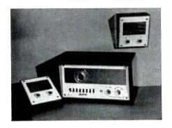
One system can be used for intercommunication between parts of offices and warehouses, and for playing background music at the same time. Each "Harmony" system consists of a master station and several
