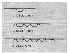
**ELECTRICAL FLEXIBILITY.** Electrical needs of today and tomorrow are easily satisfied by blending in one, two, or three cell E/R Cofar units with sections of standard Cofar.
