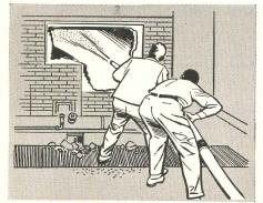
FIRE-RETARDANT. In a recent 2-hour UL fire test, Cofar became the first electrified cellular floor system (with header ducts and junction boxes in place) to earn a fire-retardant rating.
