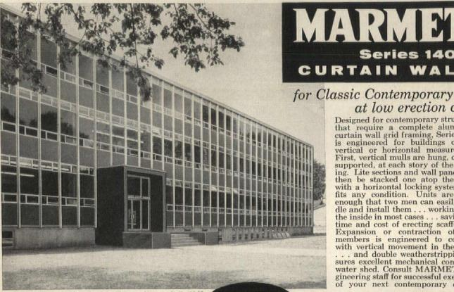
is engineered for buildings of any vertical or horizontal measurement. First, vertical mulls are hung, or base supported, at each story of the building. Lite sections and wall panels can then be stacked one atop the other with a horizontal locking system that fits any condition. Units are small enough that two men can easily handle and install them . . . working from the inside in most cases . . . saving the time and cost of erecting scaffolding. Expansion or contraction of sash
