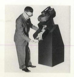
water is squeezed out and the semidry material is pushed into a container. Two or more pulpers may feed one extruder. The pulper is 30 in. high and its operation, once initiated, is automatic. Conservomatic Corporation, 113 Bala Avenue, Oreland, Pa.
