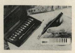
Template and Lettering Guide Pen Omnigraphos is a fountain-barrelled pen with twelve tubular nibs for ink lines from 0.3 mm to 2.5 mm in width. It is designed for use with the everincreasing number of schematic drawing templates, curve templates, and lettering guides that are presently available. The nibs are offset at an angle, enabling the user to follow guide-slot walls more closely. Laramie Chemical Corporation, 290 Main Street, Stamford, Connecticut
