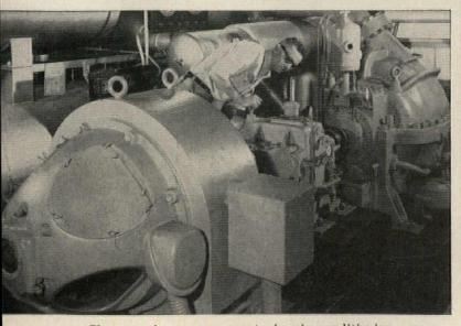
Close-up shows components in air conditioning compressor hook-up. In the foreground is a Westinghouse 250-hp wound-rotor induction motor with Type SU double-helical-type speed increaser—1760 to 6750 rpm.
