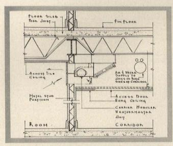
**Corridor installation** with the unit, supply air conduit and water services concealed above hung ceiling.
