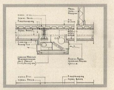
In-the-space installation where structural framing requires unit be tightly fitted against fireproof beam.
