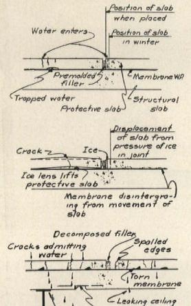
Rusting steel Pressure of rust explodes off section of conc. slob
