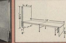
COMPACT! Each unit folds-a-way into shallow recess only 8" deep, or may be mounted on wall. Drawing shows stage folded and unfolded.
