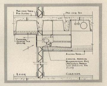
**Corridor installation** featuring twin coils in parallel mounting to attain extra high cooling capacity.
