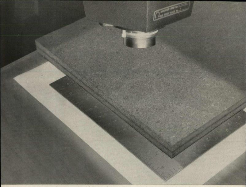
Start of test. Carpenter's square butts corner of Temlok Roof Insulation placed on sensitized paper. Strong light from enlarger strikes paper from above.
