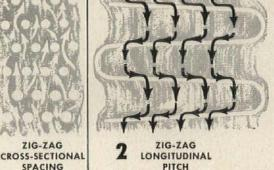
Acme's zig-zag spacing improves coil efficiency in two ways. First by staggering the tubes cross-sectionally, both air and spray water are forced to travel a longer zig-zag path through the coil effecting greater turbulence and better heat transfer.
