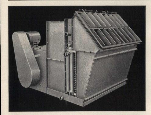
**Type AB Multi-Zone Unit** is in one arrangement for either horizontal or vertical air flow. A diffusion section is furnished between the fans and coils to distribute the air evenly over the entire face of the cooling and heating coils.
