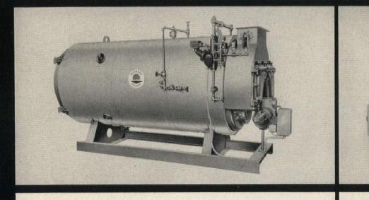
NEW 18 TO 92 HP CAPACITIES: For 125-150 swp or high temperature water above 250° F. Kewanee Scottie Jr. high pressure boiler with a Kewanee burner for oil (shown) or gas. Features include long gas travel, ample steam space, x-rayed and stress relieved welds. OTHER LARGER KEWANEE BOILERS range up to 651 hp for high pressure ... 21,855,000 Btuh for low pressure. Matching forced-draft burners are available for oil, gas and gas-oil combination firing.
