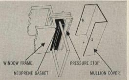
Neoprene gasket fits over glass edge. Aluminum pressure stop covers the gasket and is bolted into the window frame. Mullion cap covers the joint. Result: a tight, leakproof but resilient seal.
