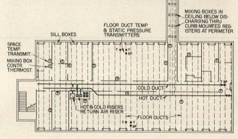
As shown in the plan at right, hot and cold air for office spaces flows through conventional risers and supply header ducts to secondary ducts in the cellular floor. Thermostats, and temperature and pressure transmitters at various points throughout the system permit accurate control
