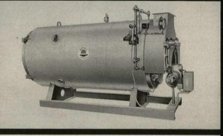
NEW 606,000 TO 3,060,000 Btuh CAPACITIES: Kewanee Scottie Jr. low pressure boiler with Kewanee burner. Firing rate is balanced with boiler capacity. Oil burner (shown) is high pressure, twin nozzle type. Gas burner is equipped for either natural or LP gas.
