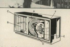
Lennox Air Processing Unit introduces fresh air in adjustable volumes (A); transmits warm air (B) from adjacent or remote heating unit; continuously recirculates indoor air (C); filters air clean (D). Lennox' exclusive floating blower (E) and acoustical lining (F) assure a degree of quietness never before achieved.
