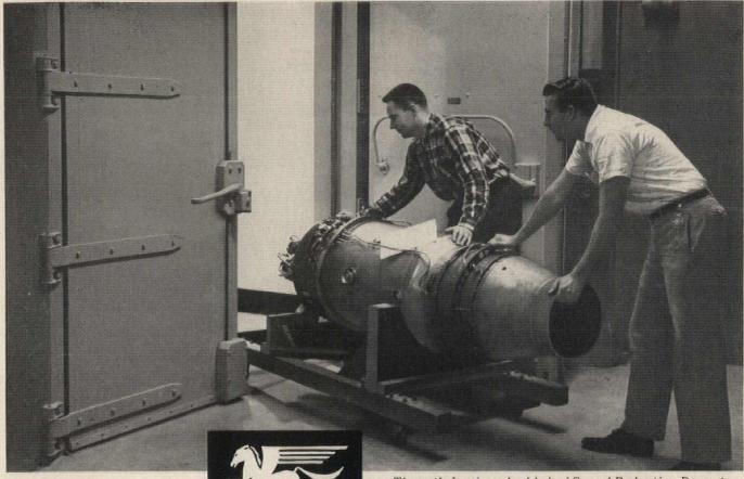
Through Jamison double leaf Sound Reduction Doors goes turbojet engine for testing. Note massive vibration proof hardware.
