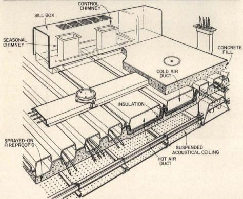
Although primary distribution is essentially the same as for conventional dual duct systems, the new Robertson system uses a cellular steel floor—which also provides electric raceways—for secondary air distribution. A major advantage is that both the hot and cold ducts can be used to carry cold air thus reducing the amount of ductwork required
