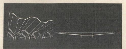
Tapered folded plate for National Airlines hangar at Miami is cantilevered-sans cablesfrom a 2-story center core. Offices are on top level; shops in open nose pockets below
