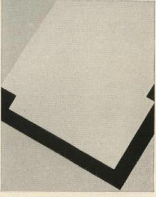
End of test. Absence of exposed line between carpenter's square and insulation panel proves corners of Temlok Roof Insulation accurately square-cut to provide firm, even base for built-up roofing.
