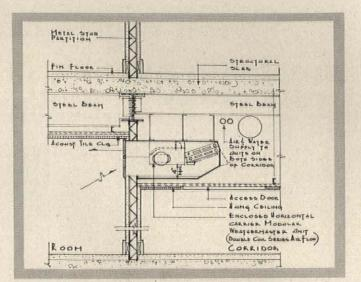
**Corridor installation** featuring twin coils for extra capacity. Enclosed unit prevents cross circulation.
