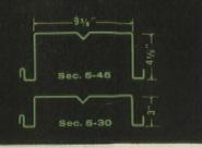
The basic cross-section of Section 5-45 and 5-30 is the same as standard long-span Section 5-75. Only the vertical dimensions are different.
