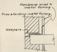
If this or something like is, is not provided, water running down the inside of the woll, will be trapped on top of the floor slab
