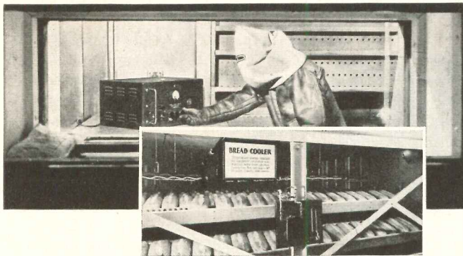
"Climate Room" (top photo) for testing electronic equipment in temperatures as low as -76 F., readily obtained with "Freon-22." Bread cooler (below) in modern bakery cuts cooling time from several hours to 80 minutes!
