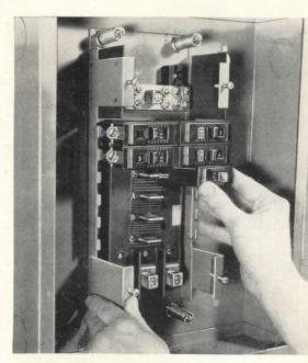
QUICK-MAKE, QUICK-BREAK PLUG-IN BREAKER—Trumbull's new NLTQ Panelboard introduces the first plugin circuit breaker with quick-make, quick-break operation. Other features: both thermal and magnetic protection... trip-free... pressure-type silver-plated copper plug-in contacts ... all ratings physically interchangeable. Adjacent breakers are on alternate phases—assuring balanced loads and circuits.
