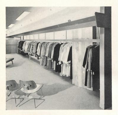
Above: air conditioning ducts are supported by patented steel struts and screened with perforated asbestos cement panels; panels are yellow, vents are bright red. Right: the architects designed dress and skirt racks and display cases
