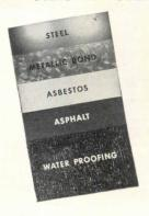
Steel sheet with asbestos felt metallically bonded to it. The felt is then impregnated with asphalt and waterproofed. The bond is inseparable, to all purposes forming a new kind of material. Maroon, black or aluminum color; fabricated in a variety of shapes.
