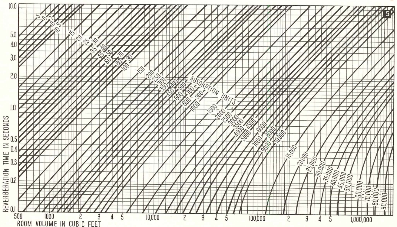
5. Chart for calculating reverberation time or sound absorption of a room
