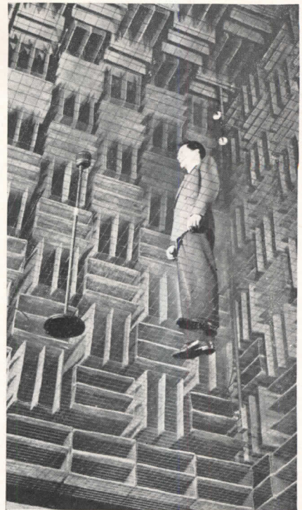
Special acoustical room is designed for complete sound absorption. Work floor is steel net suspended in space
