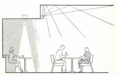
Above, left: in Hutton's bar ''pin-hole'' projectors, centered over table and bar tops, give areas of intimate 'isolation.' In main dining room, right, coves supply chief light, with two chandeliers for sparkle. Lowered area, under ducts, has ''pin-hole'' system. In plan, R represents pin-holes; S, surface mounted; U, indirect urns. H. H. Siegel, Architect; E. D. Rapp, Designer. Thomas Smith Kelly, Lighting Consultant
