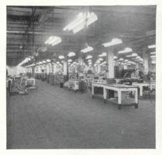
In general factory areas, industrial asphalt tile provides a durable, economical floor that's fast trucking, nonslip. Unlike troweled-on types of flooring, industrial asphalt tile can be put into use immediately after it is installed.
