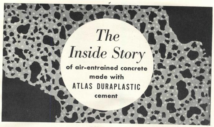
A highly magnified section of Duraplastic concrete would look something like this. The two large black areas represent small portions of coarse aggregate; small black spots represent sand; gray area represents cement paste; white dots represent entrained air bubbles.
